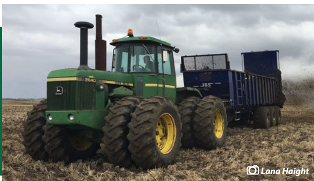
LFCE employee Roger Janzen spreads manure from our feedlot on a barley field, south of Clavet. Equipped with GPS and continuous load weighing, the precision spreader applies the manure at known and variable rates, based on soil fertility and crop yield data.
